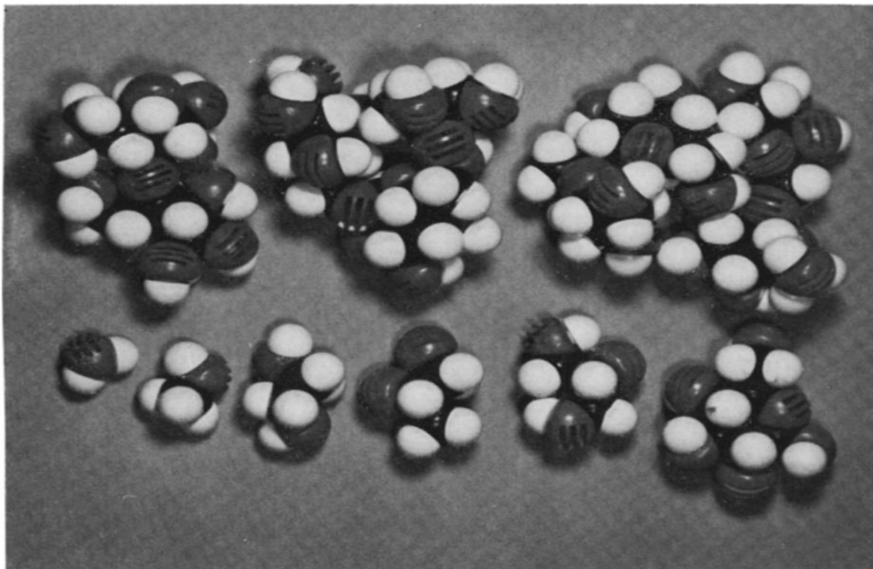
Fig. 2. CPK molecular models used to determine the unhydrated radius of calibrating molecules. In the order of their increasing size, the models represent water, methanol, ethylene glycol, propylene glycol, glycerol, and glucose (bottom row); maltose, raffinose, and stachyose (top row).
